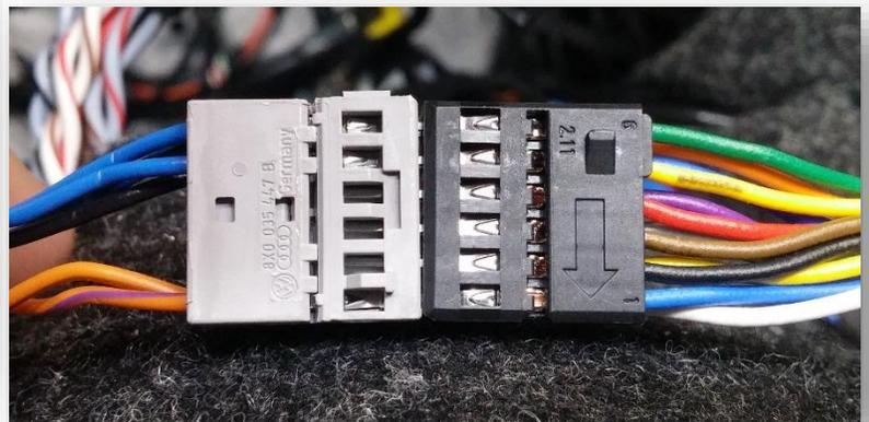
Connect the female 12-pin side of the plug & play portion to the OEM main quad-lock connector as shown. **Note the paint dot must face towards the power wires.**
