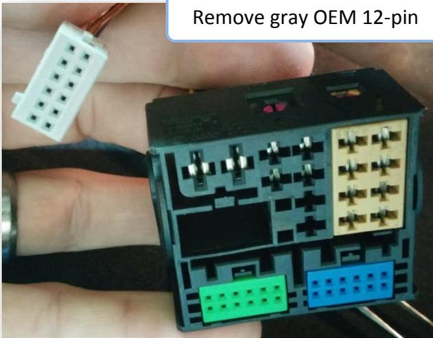
Connect OEM 12-pin to provided 12-pin (black, PIN-side). **NOTE: blue and green wire corner locations on provided plug vs OEM.**
