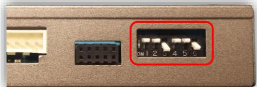
**Note:** Remove power to the unit prior to making adjustments to the dip switches.
