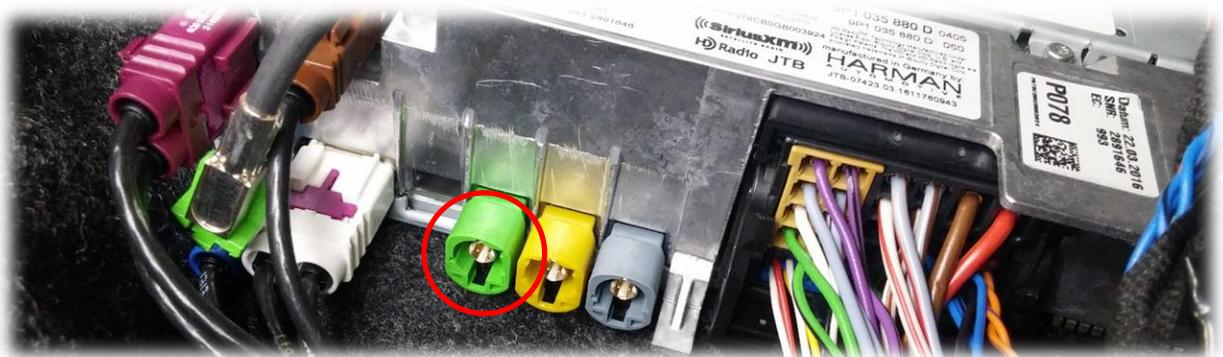
4. Connect the smaller white plug side of the provided **LVDS Video Cable** to the port on the PCM4-CAM interface labeled **VIDEO-IN**.
