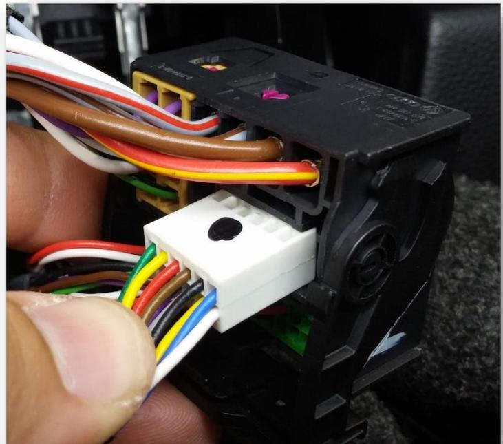
7. Connect ground and power for your camera (use an ACC source for power) and run to the front of the vehicle.
