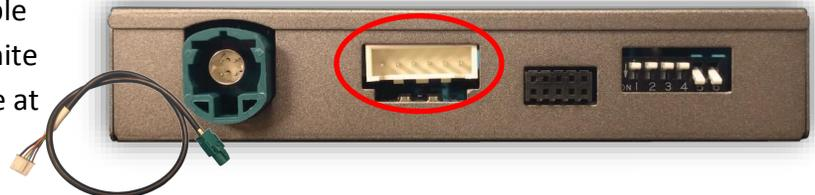
7. **Optional:** Connect the provided Reverse Trigger Input cable to the UConnect-RVC interface at the plug labeled 'CAN2' **only if CAN data does not trigger the reverse screen properly.**
