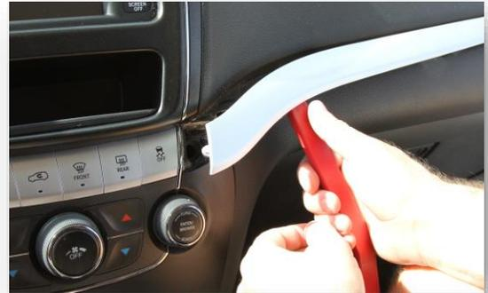
2. Remove (2x) Torx 20 screws that secure the HVAC control panel. Remove the HVAC control panel, disconnect all harnesses and set it to the side.
