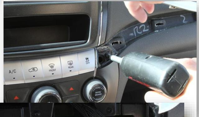
3. Remove (4x) Torx 20 screws which secure the radio stack into the sub-dash. Remove radio, disconnect all harnesses and set it aside.
