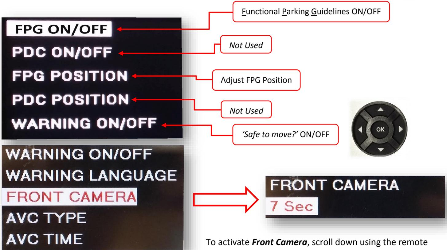
To activate **Front Camera**, scroll down using the remote arrow keys when in the menu to **FRONT CAMERA**. Once in this setting, press OK and choose (up/down) between 5, 7, 9 or 11 seconds for **auto-front switching timeout** (once the vehicle leaves reverse gear, the front camera input will stay active for pre-defined amount of time).
