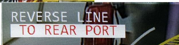
To set custom **green wire trigger**, find 'REVERSE LINE' option and set to 'REAR PORT' or 'AV1' depending upon your preference. Every time the green wire receives 12v (+), the selected RCA port will display on screen.
