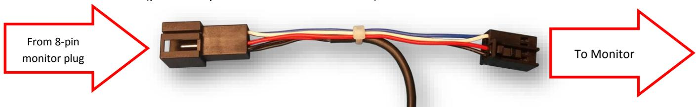
**NOTE:** You may have to shave the keyway of the OEM connector to fit it into the female side of this connector for some vehicles.
