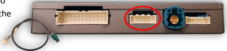
5. Connect the provided Plug & Play T-Harness (CAN/Power) to the screen, from the blue connector (previously connected to the screen).
