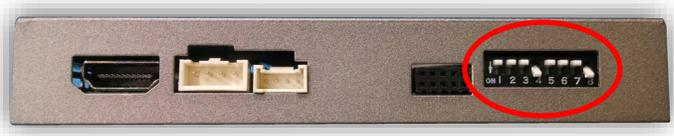
**\*Note: Remove power to the unit prior to making adjustments to the dip switches.**
