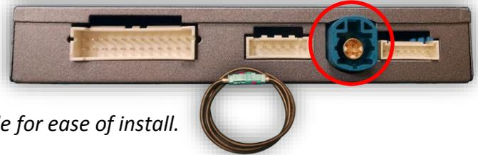
4. Connect the *provided* LVDS Video cable to the OEM monitor (green plug). Connect the other (white) end of this cable to the W204-N interface here:
