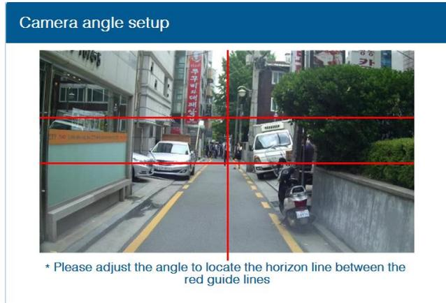
In case of indoor installation or somewhere you cannot see the horizon properly, use same data to "**Camera Height**". Mark the same height on the wall apart about 3 ~ 5 meters from the vehicle.
