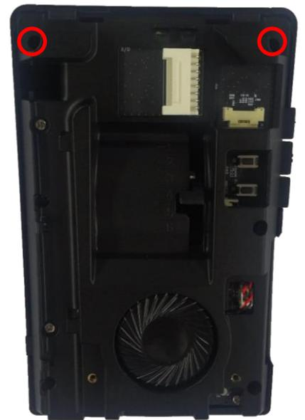
③ Remove PCB unit from mounting frame completely.
