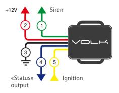
To connect VOLK module, connect its wires the following way:
