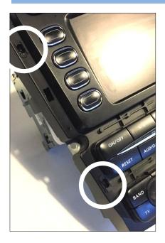
Remove the 4 x trim clip from original ZAB unit and clip into the supplied fasica
