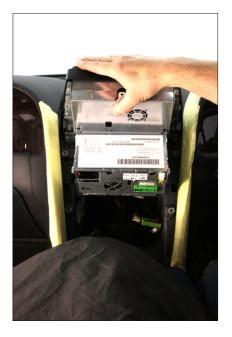
Disconnect all connections to factory radio and remove from car.
