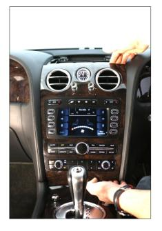
Take hold of the trim panel and pull from the top and the bottom to remove
