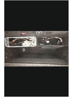
Remove the navigation drive and the CD changer to make it easier to run the supplied GPS extension lead.
