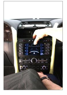
Carefully remove the Bentley head unit
