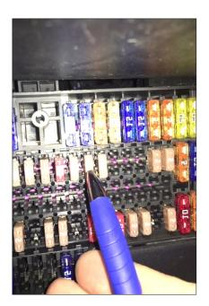
Remove the 5 amp fuse in location 28 for the phone module
