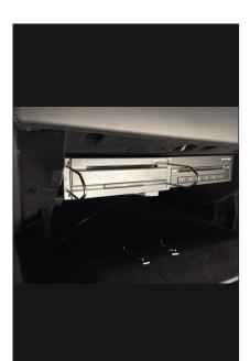
Disconnect the Navigation CD drive in the glovebox.
