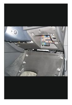
Remove the fuse for the phone module. Locate the fuse board in the driver side foot well
