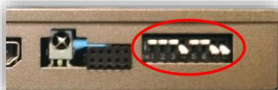
**Note: If the dip switches are not configured prior to installation you must remove power to the unit prior to making adjustments to the dip switches.**
