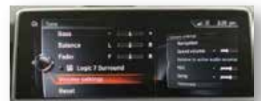
Logic 7 controls the 2 different time alignments*
