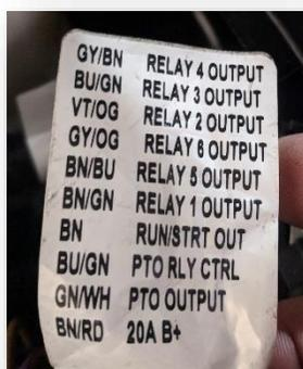
*UpFitter switch wires (engine bay drivers side near firewall)*
