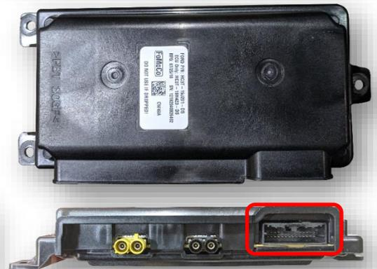
4. Connect the 8-pin harness from the main T-Harness to the SAT-switcher board's 8-pin port.
